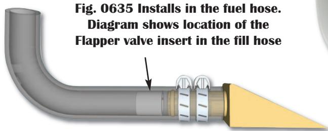
**Fig. 0635** installs in the fuel hose. Diagram shows location of the Flapper valve insert in the fill hose
